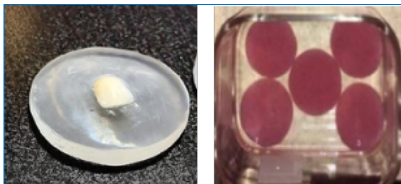
Figure 1. (A) Denture tooth in a specific acrylic jig. (B) The acrylic resin specimens were immersed in denture-cleansing solutions.
