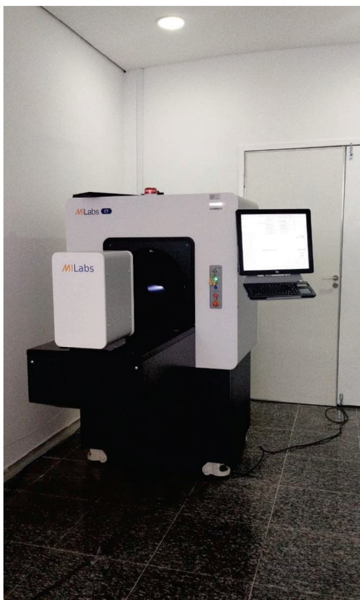
FIGURA 01: VISTA GERAL DO MILABS U-CT IN VIVO DIAGNOSTIC PRECLINICAL X-RAY CT SCANNER (MICROTOMÓGRAFO).
